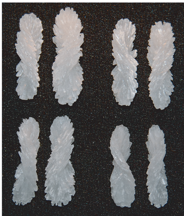
Figure 6. The macroscopic helicity of threonine aggregates reveals their predominant molecular chirality. Aggregate size: circa 15 × 3 mm.
